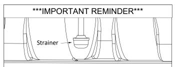
Occasionally check strainer screen to ensure it is clean and clear of any debris. Strainer is located on the end of the intake hose, inside of the tank. Use protective gear when removing hose from tank and cleaning the strainer.
